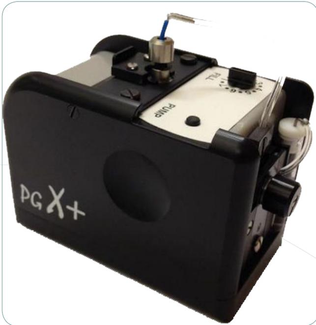
The PGX+ is a compact instrument that measures wetting and absorption on virtually any size or shape surface without the need to cut sample strips required by other contact angle testers.
