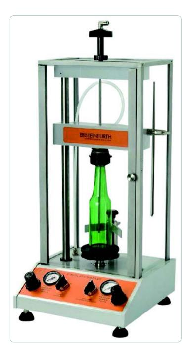
The Steinfurth Sampler pierces and pressurizes bottles and cans. Piercing and sampling is performed pneumatically, so there is no need for great manual forces. Fully automatic operation makes beverage sampling even very simple. The Steinfurth Sampler is suitable for gas analyses (e.g. oxygene, CO2,...) and foam stability measurements.
