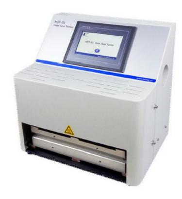
Heat Seal Tester is applied in measuring heatsealability of a surface, or sealant layer of films, laminates, composites and polymers etc. How well the material heat seals is expressed quantitatively as seal strength as a function of the sealing conditions
