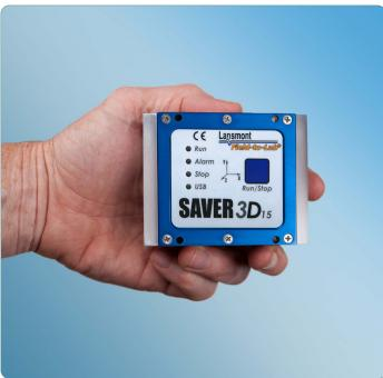
SAVER™ 3D15 is a self-powered field data recorder with an internal tri-axial MEMS accelerometer, possessing DCresponse measurement capability. The 3D15 also incorporates temperature and humidity sensors, and USB connectivity. Powered with 9V lithium batteries, the instrument will operate continuously for up to 15 days. 16-bit resolution allows you to take precise measurements of your dynamic environment.
