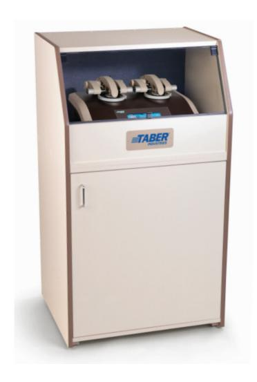
The typical sound level of operating a Taber Abraser and its vacuum system can exceed 80 dB. Utilizing sound deadening materials, the Quiet Cabinet reduces the audible level up to 21/2 times (20% reduction in decibels) and provides a noise level comparable to a standard office environment. Constructed of laminated particleboard, the Quiet Cabinet includes a high-pressure laminate outer shell which provides added durability and blends with any laboratory or manufacturing environment.
