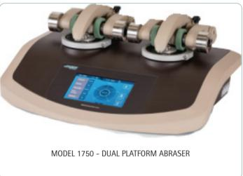
"Taber Test" delivers reliable data in minutes. Used to evaluate a material's resistance to wear, a flat specimen is mounted to a turntable platform that rotates on a vertical axis. As the turntable rotates, contact of the specimen against the sliding rotation of two abrading wheels cause wear while a vacuum system removes loose wear debris during the test. The resulting abrasion marks form a pattern of crossed arcs in a circular band that cover an area approximately 30 cm<sup>2</sup>.
